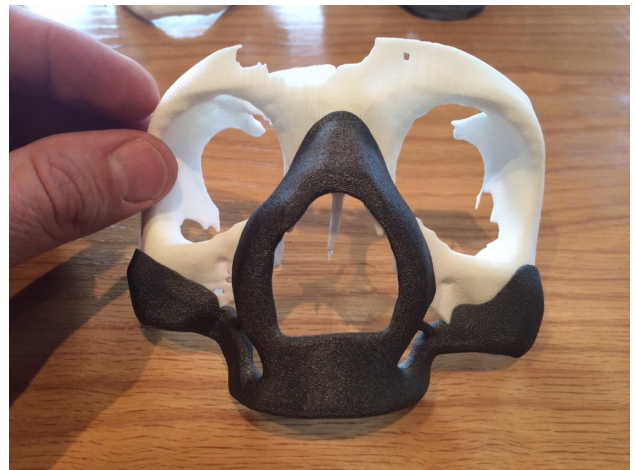
Fig. 4. Demonstration of how the 3D printed nylon prototype fits onto the planning model.
